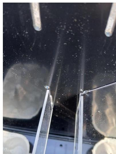
5. Attach the light-board (which is where the bulb sits) by slotting the tabs on the horizontal plastic base of the light-board into place. These grooves are the large grooves located above the grooves where the thin Perspex strips slot into place.
