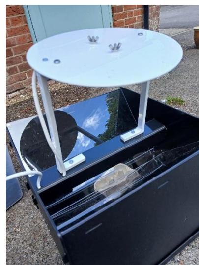
6. Carefully screw the bulb into the lightboard so that it hangs down over the moth trap. **Ensure that the moth trap is NOT attached to the battery at this stage.**
