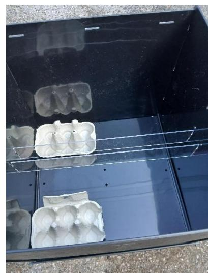
4. Take one of the large pieces of Perspex and position so it is sloping inwards towards the middle of the trap. Slot into the appropriate groove (small hole above where the parallel strip of perspex clips in). Repeat opposite with the other piece of Perspex so that they are both sloping down towards the middle of the trap.
