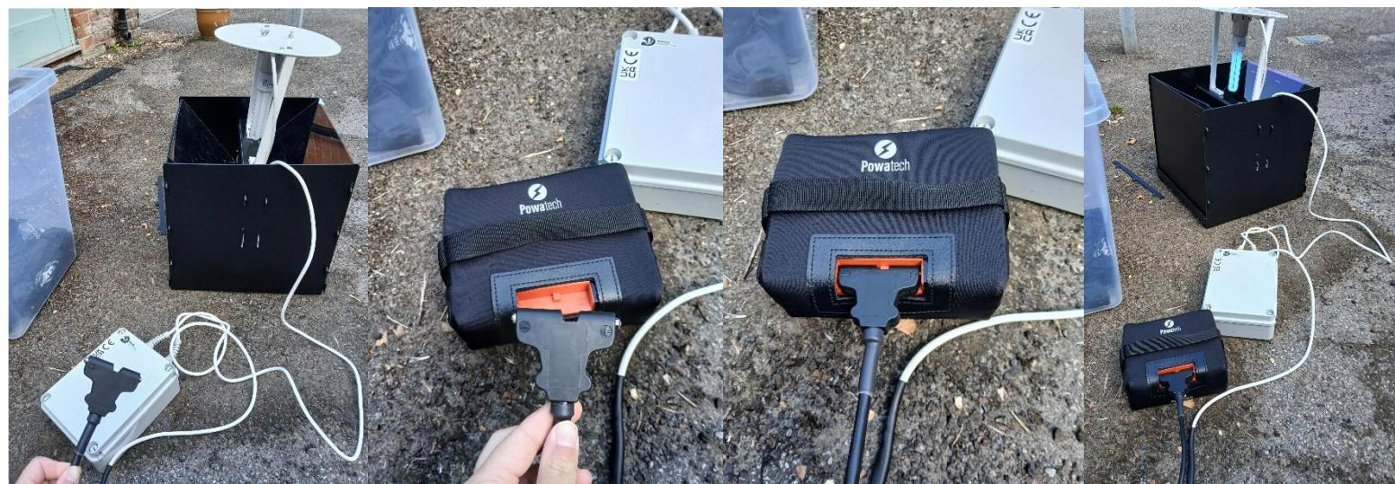
13. Before leaving the trap, if it is due to rain place the battery in the plastic box provided. The lid can be placed loosely on top to allow the wire to come out. This will help protect the battery.,
